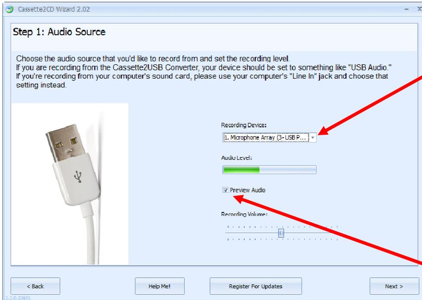
Select the Recording Device, in this case the "USB Audio" option.
